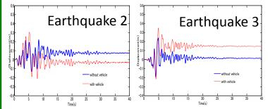
The maximum rotation in the hysteresis loop of the bridge with vehicle is larger than those without vehicle, indicating the bridge suffered from a more severe plastic behavior.
